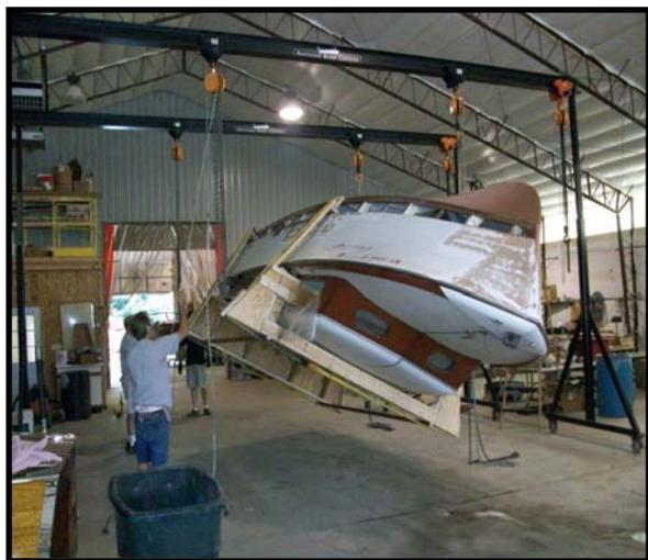
After the bottom was removed we discovered far more structural damage than any of us expected. After replacing most frames, chines, gripe, stem and keel repair we installed a new cold molded bottom. Bob's son Pat worked with us throughout the entire project and was a huge help both with the work and answering any questions had about the history of the boat's usage. The boat should now perform long into the future.
