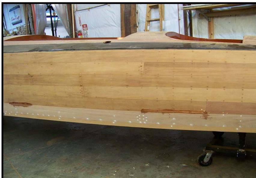
*Between each coat (10-12 coats) the boat is sanded in preparation for the final coat of varnish.*
