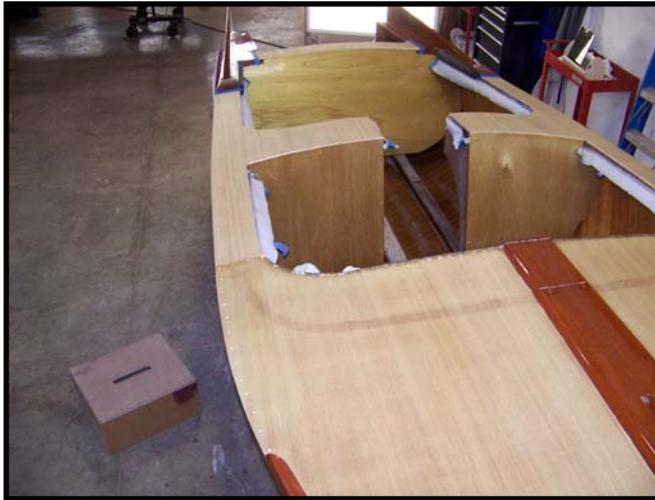
This boat is a 1957 15' North American O/B. The owner, Ron Hooker, has owned the boat since new. Ron brought the boat to us for new decks/covering boards and partial refinish. We replaced the front seat backs and rear seat back/bulkhead. Also replaced were the battery and fuel tank hold down. The exterior gets fresh paint and varnish.
