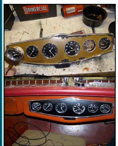
Rick Roy purchased his 1939 Chris Craft 19' Custom from us last fall. He chose to leave the boat with us for some work over the winter. We flat sanded the boat to remove finish imperfections then varnished the boat, replaced the manifold, installed a new fuel tank, all new fuel system, re-wired the boat, cleaned up the gauge cluster, and applied a gold leaf name. He plans to pick up the boat next weekend.
