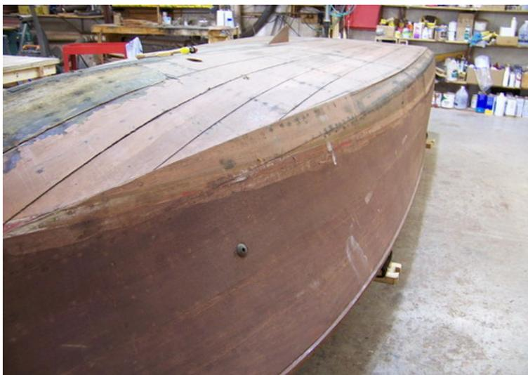
*The initial inspection of original bottom shows significant plank separation. This boat currently is unusable. It will be restored with a water-tight cold molded bottom.*
