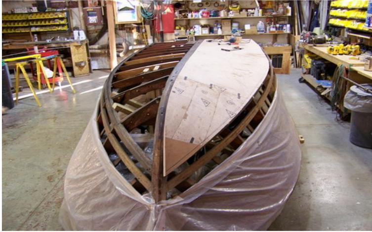
*Original oil soaked bottom planks have been removed and frames replaced as needed. Cold molded shells will be fitted in preparation for the new cold molded bottom.*
